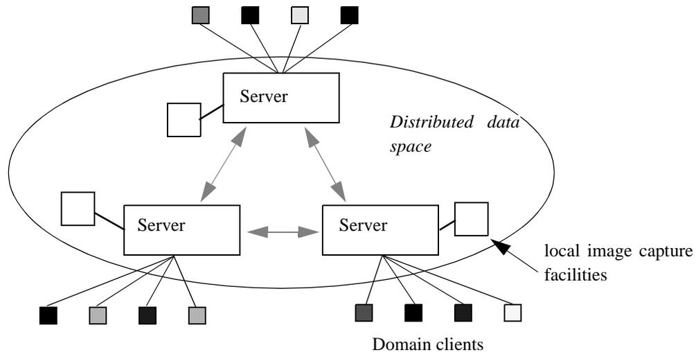
**FIGURE 2. The structure of the Portholes system. Portholes consists of a number of cooperating information servers linked by a network. Client programs communicate only with their local servers, although they may display remote information. Servers use local image-processing facilities.**
