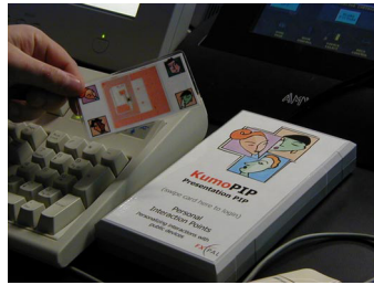
Fig. 4. A user logs into an embedded PIP interface by swiping an RFID card.
