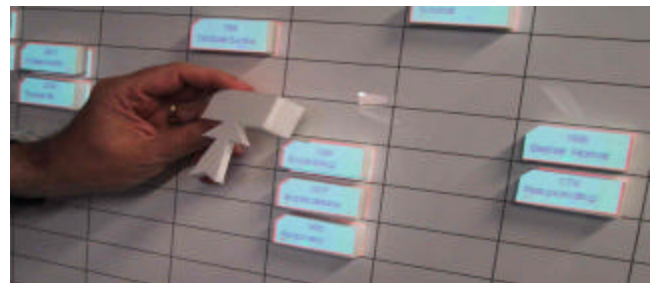
Figure 4. “Group” command: The user is about to execute the command by placing its command puck (with the arrow) over the topmost data item of the column to be grouped. The items will then be grouped into a single item, at the location of the command puck.
