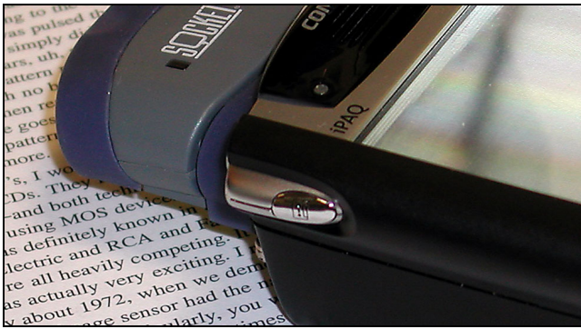
Figure 4. The trigger button initiates bar-code scanning.
